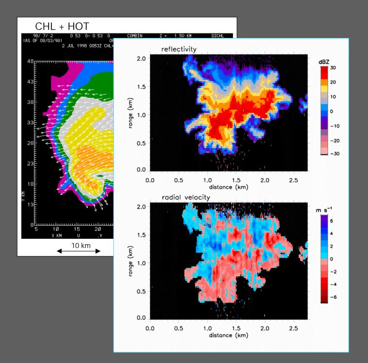
Increased resolution compared to ground-based radars, and the flexibility to move to selected clouds are the main advantages of airborne cloud radars. Limitation to vertical and horizontal planes, and attenuation, are the disadvantages. Attenuation does not influence the derived motion fields.
