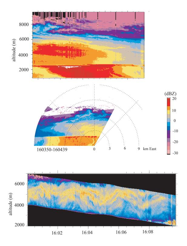
Fig. 9. Radar equivalent reflectivity images for Sept. 6, 1995. The top and middle panels are images from the NOAA K<sub>a</sub> band radar. The top panel is for vertically pointing beam and the middle image is an RHI scan at  $270^{\circ}$  azimuth. The bottom panel shows data from the airborne radar (WCR) during the spiral descent; see the text for an explanation of this display.
