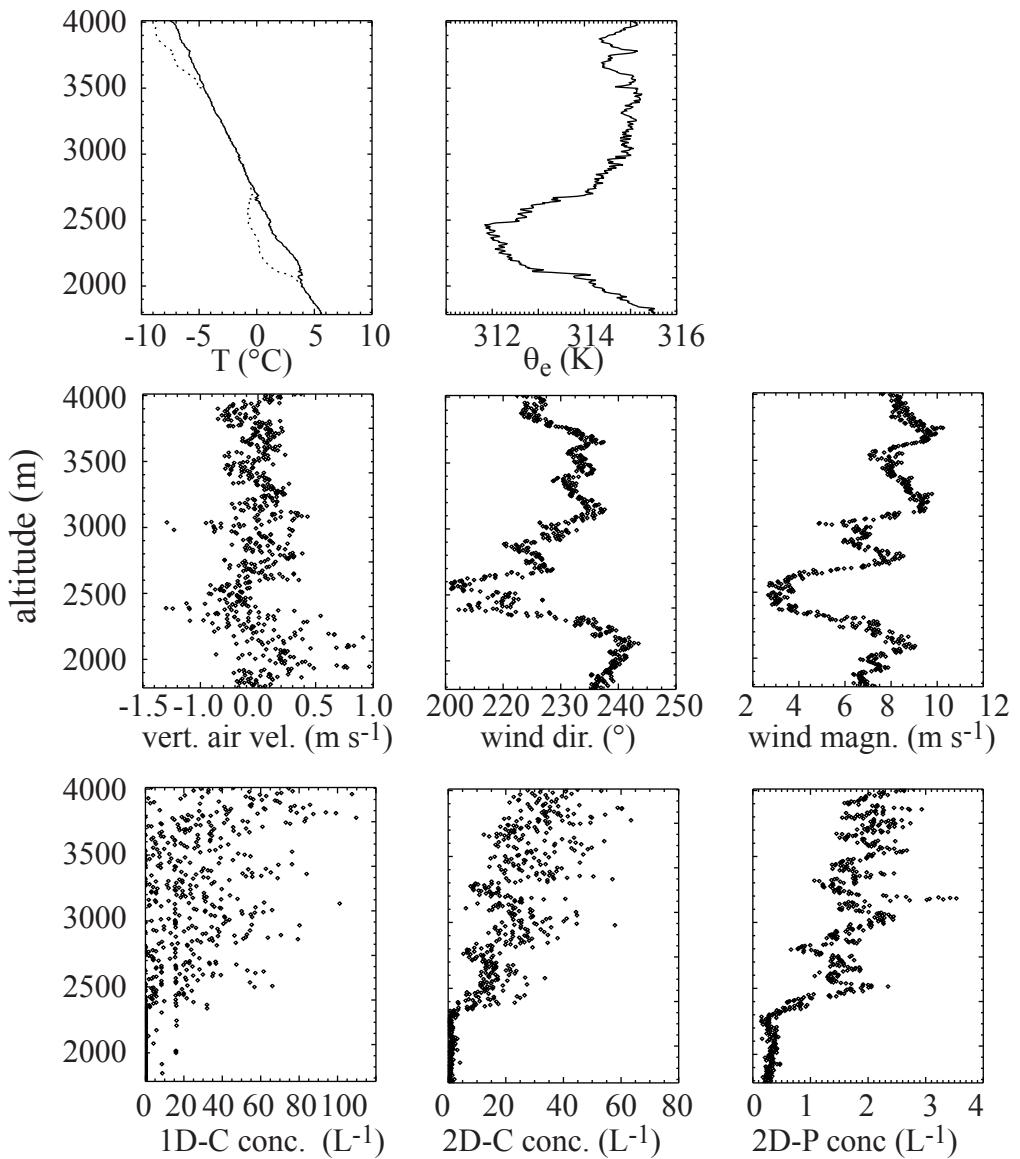
Fig. 10. Vertical profiles of different parameters during the spiral ascent on Sept. 6, 1995. The dashed line in the first panel is dew point temperature.
