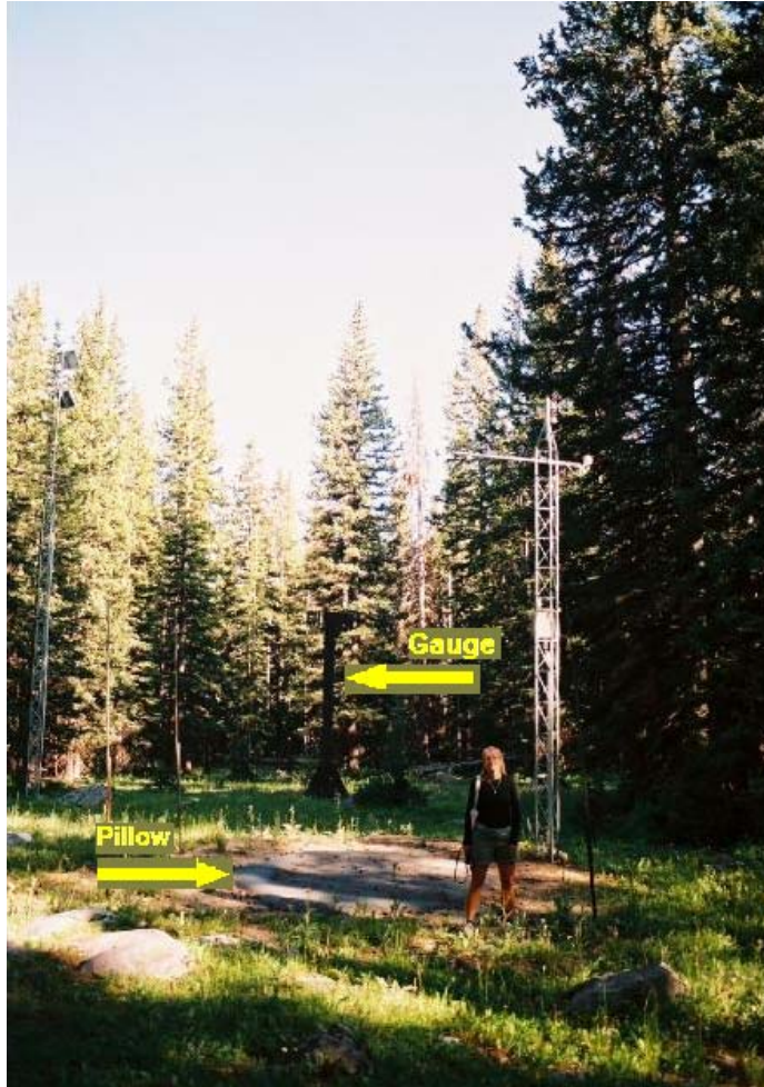
Figure 3.6 - Snow pillow and the Alter-shielded gauge sensors at SNOTEL. The pillow measures the snow water equivalent of the wintertime snowpack.
