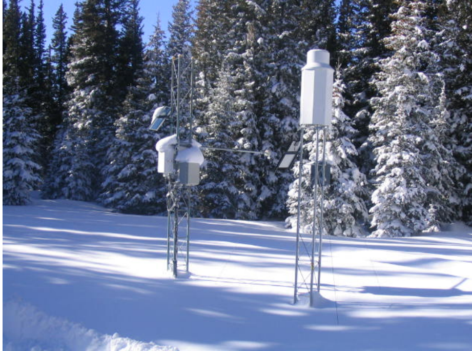
Figure 3.7 - Vaisala Rain Gauge (right) operated by NCAR at the GLEES site during 2007 and 2008.
