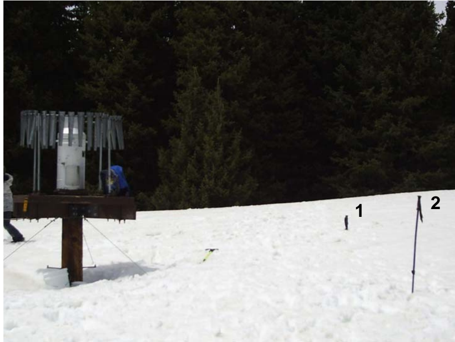
Figure 3.3 – Snow depth measurements made near the NADP-gauge at the GLEES. Picture is taken on 20080519. At left is the Alter-shielded NADP-gauge. To the right there are two probes inserted to the soil surface indicating the snow depth increases ~1 m in a horizontal distance of ~3 m. The probes were positioned along the dashed line shown in Figure 3.2.
