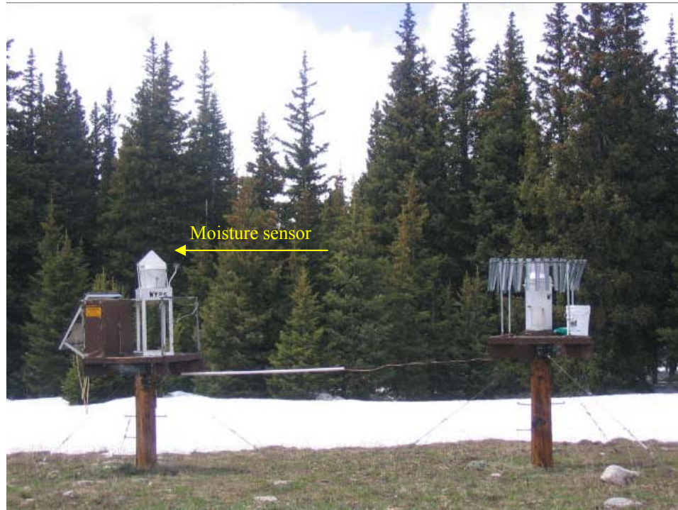
Figure 3.5 – Brooklyn Lake NADP site located at the Glacier Lake Ecosystem Experiments Site (GLEES) in the Medicine Bow Mountains of southeastern Wyoming. On the left is the sample volume sensor and on the right the Alter-shielded Belfort precipitation gauge. (Picture is taken 20070521)
