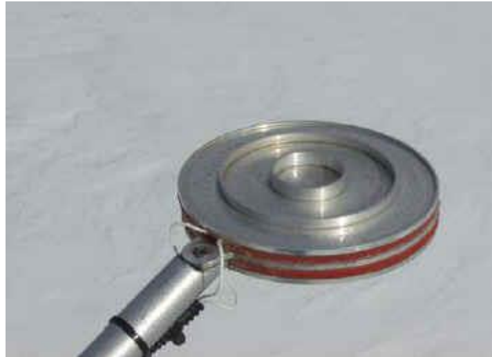
Figure 1 – The Yankee Environmental Systems Hotplate Precipitation Sensor ( http://www.yesinc.com/products/data/tps3100/index.html ).
