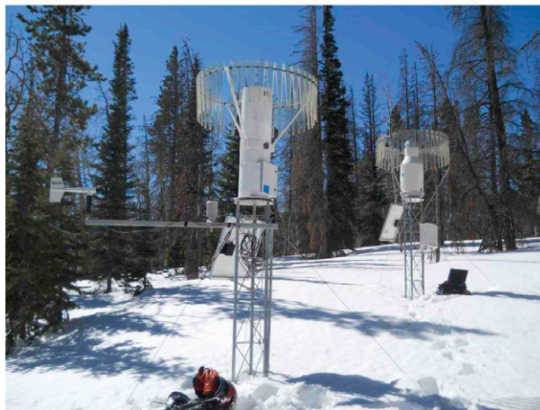
FIG. 5. Photographs show the deployment of (top) a ground-based AgI seeding generator in the Medicine Bow Range and (bottom) precipitation gauges in the Sierra Madre Range.
