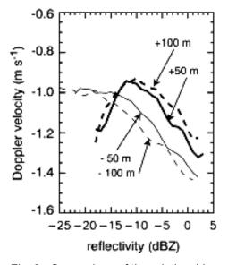
Fig. 2. Comparison of the relationship between reflectivity and Doppler velocity at different altitudes near cloud base.
