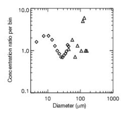
**Fig. 1.** Ratio of drop concentrations in the 80<sup>th</sup> percentile of vertical velocities to drop concentration in the lower 20<sup>th</sup> percentile of vertical velocities.
